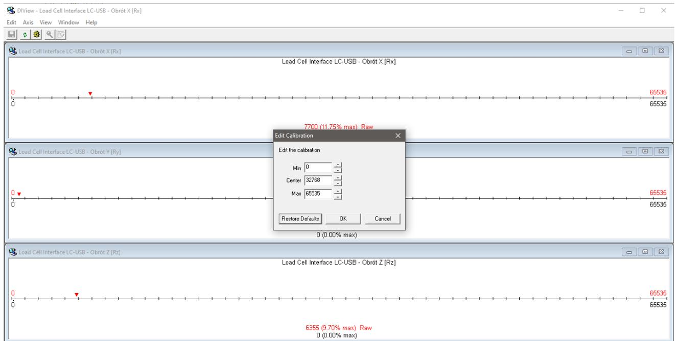
5. In the calibration, we consider only the red numbers the X-axis pedal at rest is 7700. Add about (300 to 500) to this number and enter in the MIN box
