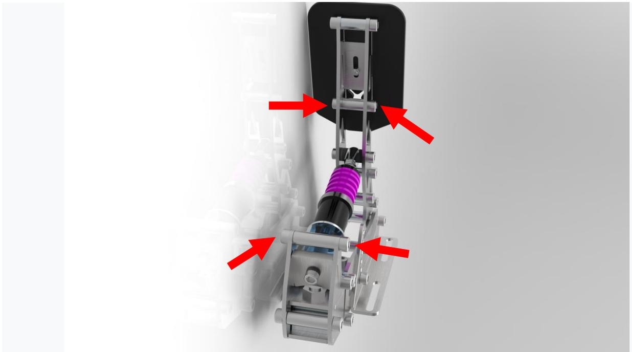
a) Remove all screws marked with red arrows and remove them metal bushings
